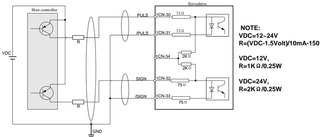
**Note:** When the host controller is applied by open-collector signal output, the input signal noise margin lowers. When a
