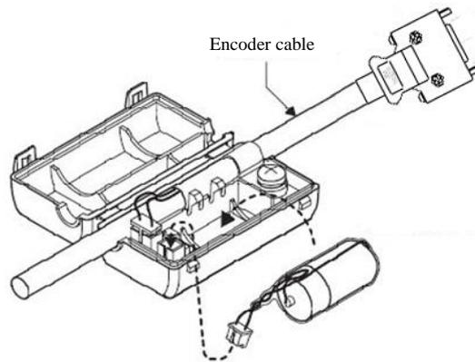
C. Cover the shell of the battery case.
