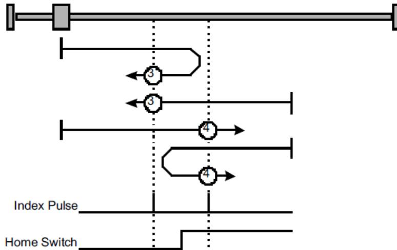
**Methods 5 and 6: Using negative reference switch and zero impulse evaluation**
