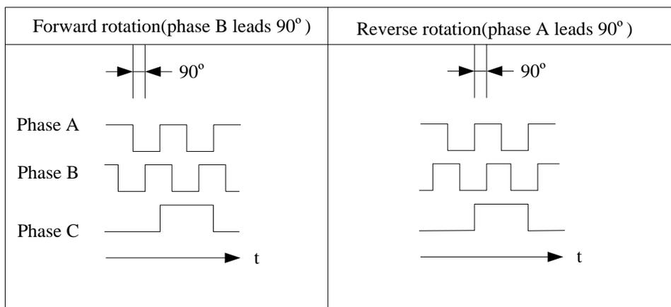
If the Servo motor is not equipped with an absolute encoder, the Servo motor needs two full rotations before using the servo drive's Phase-C pulse output as the zero point reference.
