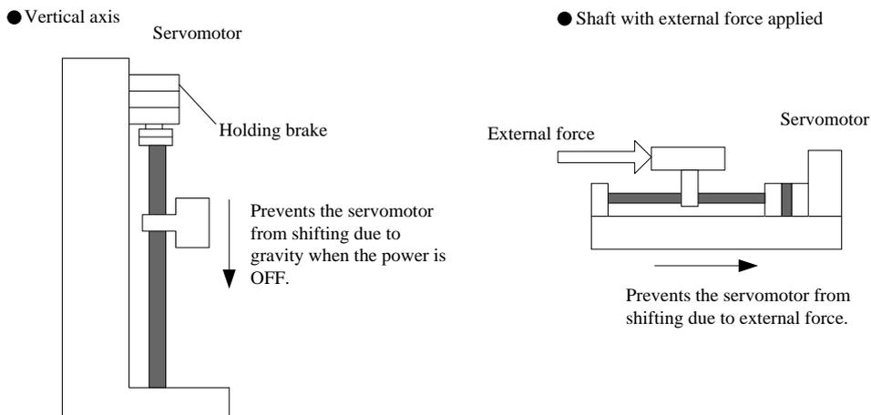
1. The Servo motor with the built in brake, is a de-energization brake. It is used to hold the Servo motor and cannot be used as a braking purposes. Use the holding brake only to hold a stopped Servo motor.
