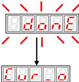
5. Press the ENTER key to return to the utility function mode display Fn005.
