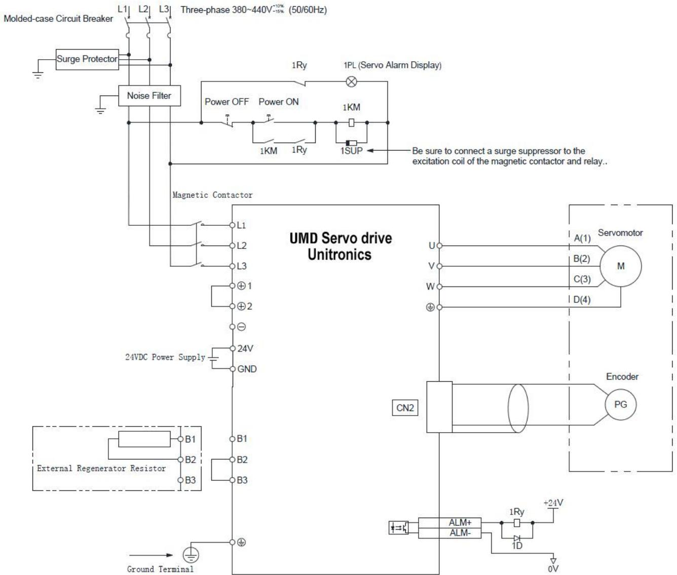
The I/O signal connections diagram of the UMD-□□-E3 servo drives is as shown in the following figure.
