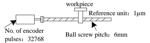
To move a workpiece 10mm using reference units:
