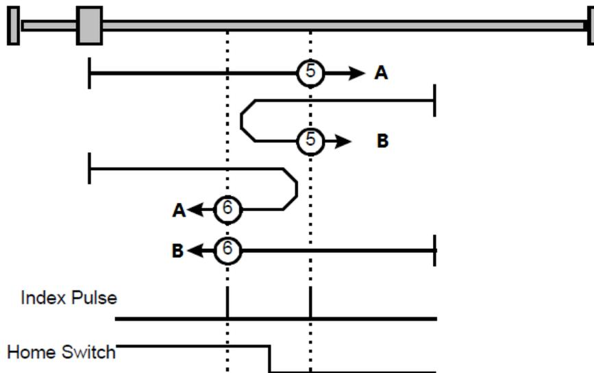
**Methods 7 ~ 14 Using reference switch, limit switch and zero impulse evaluation**
