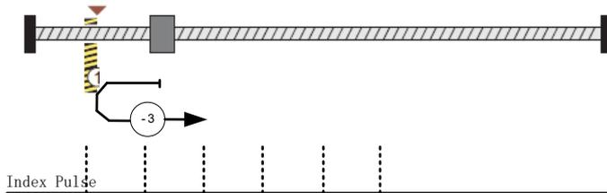
**Method -2: Movement in positive direction, hitting an end, makes the current position for the origin.**
