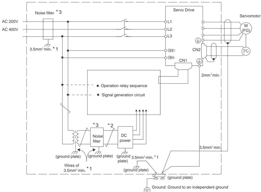
•For ground wires connected to the ground plate, use a thick wire with a thickness of at least 3.5 mm<sup>2</sup> (preferably, plain stitch cooper wire)
