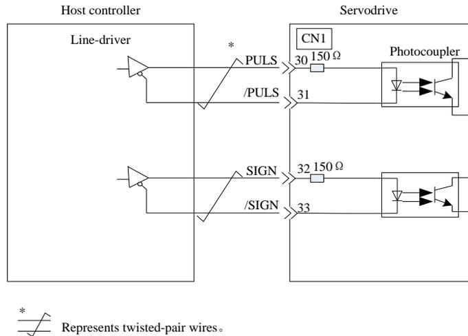
(b) Connection Example for Open-Collector Gate Output
