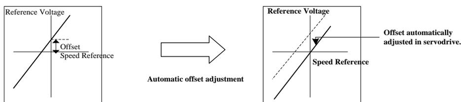
After completion of the automatic adjustment, the amount of offset is stored in the servo drive. The amount of offset can be checked in the speed reference offset manual adjustment mode (Fn004). Refer to **4.5.3 (2) Manual Adjustment of the Speed Reference Offset**.
