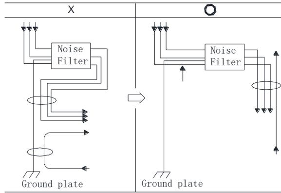
Install the noise filter shield directly to the ground plate. Do not install the noise filter to the painted control panel.
