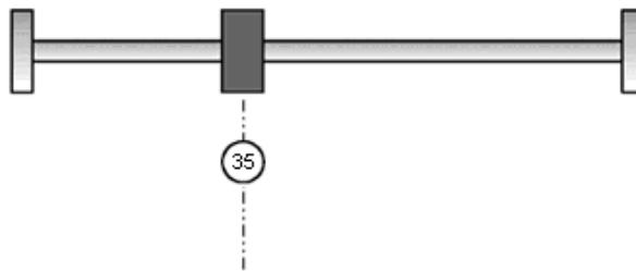
**Method -4 Movement in positive direction, hitting an end and reversing to travel, the target homing position is the first C pulse**
