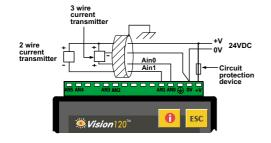
7. Shields should be connected at the signals' source.
