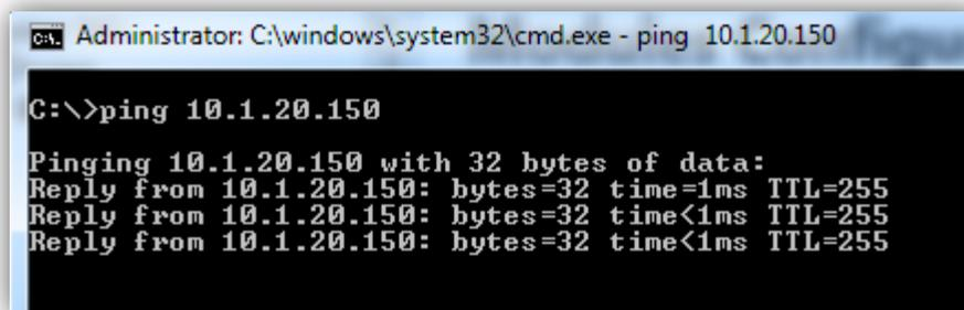
12. If the adapter replies successfully, then power off the adapter (URB-TCP) and lower DIP switch #9 (set to OFF).
