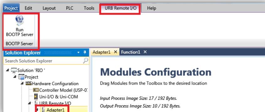
5. Click Start BootP in the **Unitronics** BOOTP Server; the upper section displays Ethernet devices that are in the network.
