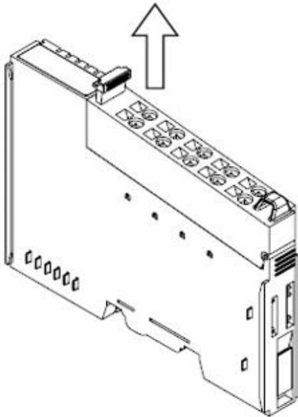
2. Apply more force until the I/O module is pulled away from the I/O module.
